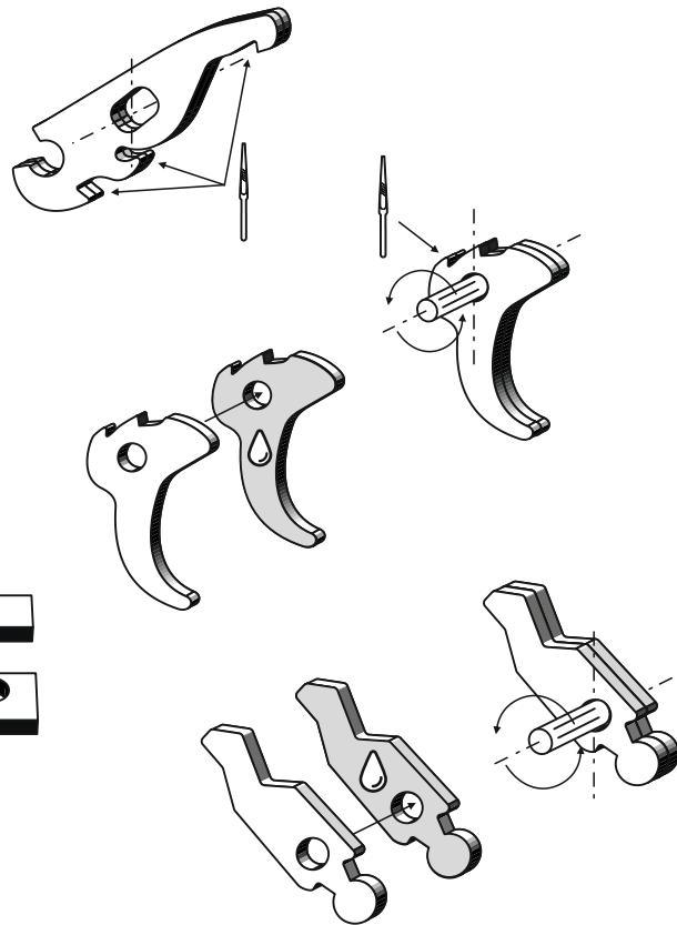
! When gluing parts, make sure that the **glue** does not get on the pin.
